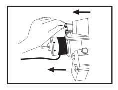
5. Slide both screw bungs out. Now slide the tubular motor out. Keep them in a safe place, you will need these later on.
