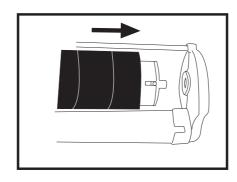
15. Slide the roller/fabric back into the frame. NOTE: Check to make sure the awning arms are still tied up so they wont get in the way.
