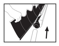
**16.** Slide the valance back onto the valance bar. Also insert the the motor into the roller.
