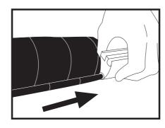
14. Once fully rolled up, slide the end of roller back into the valance bar. NOTE: Make sure the end fabric (circular part) slides into the metal (valance section)
