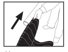
11. Replacing awning fabric cover. Slide the fabric back into the roller (find the groove)
