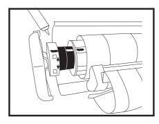
2. Use a pen, mark a straight line for reference: the lid, motor and roller. This is to make sure the awning is installed in an exactly the same position.
