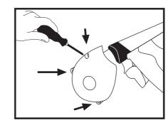
3. Remove the three screws located at side awning (lid). NOTE: usually hidden under a sticker.
